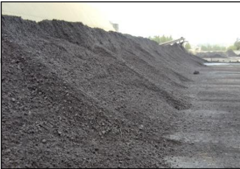
Stockpiled coal, used as the main fuel for firing the kiln, is currently being supplemented by wood waste.
