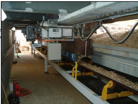
The wood waste screw, pulling wood waste material from the hopper onto the conveyer.
